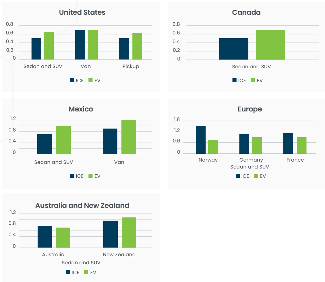
Exhibit 9: Total cost of ownership (USD) per mile for ICE and EV by geography
